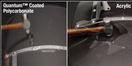
We applied a ball peen hammer at full force to one of our polycarbonate shields (left) and to a competitor's acrylic shield (right). Remember – we're professionals – don't try this at home!
