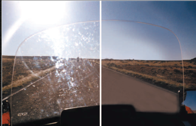
Here we see a motorcycle windshield with typical surface wear and abrasions. This is not what you want in front of you when facing oncoming traffic!
