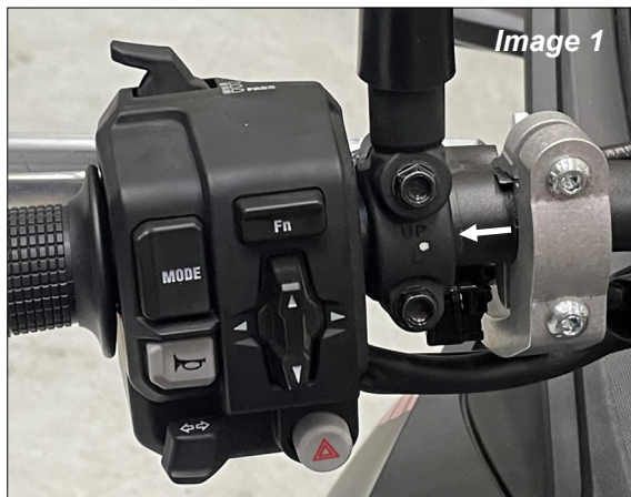
← Clamp location on handlebar
